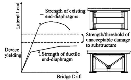
Fig. 5. Inelastic behavior of ductile end cross frames compared to existing strong diaphragms
