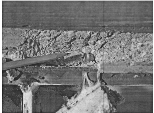
Fig. 6. Failure of shear connectors in bridge model during transverse cyclic loading
